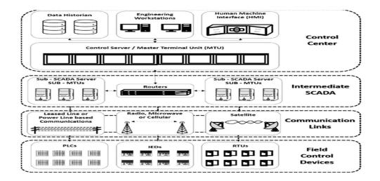
machinery for centralized monitoring and system control those on a power plant require hundreds of field devices and dedicated subsystems to reduce the load on the centralized server.
